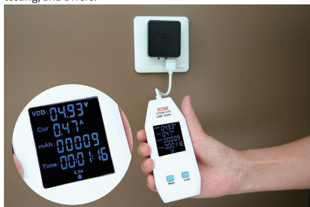
Tester with electronic load (UT658 LOAD)
