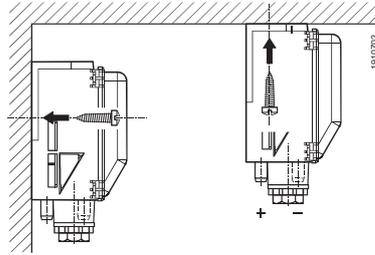
If the pressure connection nipples point upward or are at a lower level than the air duct probes, condensation can collect inside the sensor, causing damage to the device.
