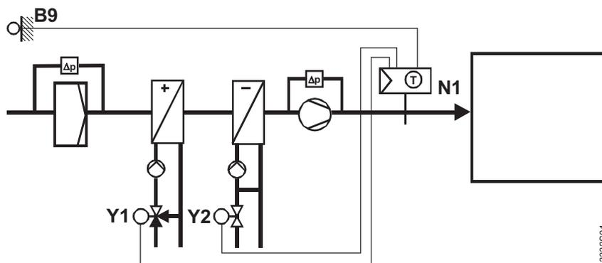
Supply air temperature control through control of the heating or cooling valve in sequence, with outside temperature compensation
