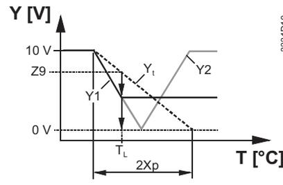
**1-stage heating and 1-stage cooling**
