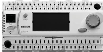
Controller/RMB795/RMS705 with operator unit plugged in
