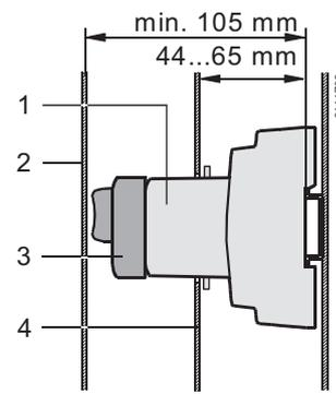
Controller/RMB795/RMS705 complete with attached operator unit is mounted inside the control panel; the operating elements can be accessed only when the control panel door is opened (internal operation).
