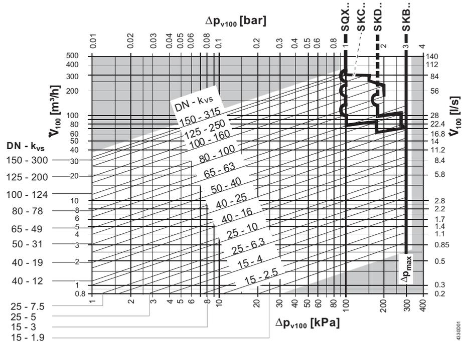
$\Delta p_{max}$  = Maximum permissible differential pressure across the valve (mixing: port A-AB, B-AB; diverting: port AB-A, AB-B), valid for the entire actuating range of the motorised valve
