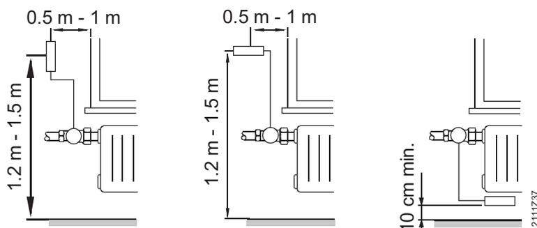
When mounted on poorly insulated outer walls, a thermally insulating layer should be fitted in between.
