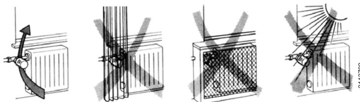
The actuator must not be fitted in the upright position to ensure that measurement of the room air will not be affected by rising air from the hot water pipe.
