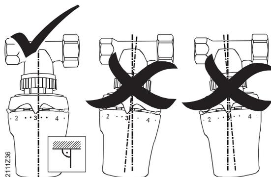
When mounting the actuator to the valve, ensure that valve and actuator form a right angle.
