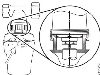
For that, select scale number 5 and ensure that the actuator rests correctly.
