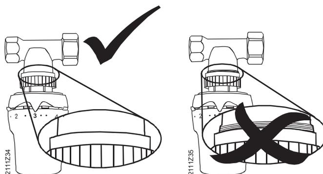
Then, tighten the actuator correctly.
