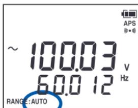
When the manual range is set, pressing **AUTO RANGE** for at least 1 second changes to the auto range. The instrument automatically selects the optimum measurement range.
