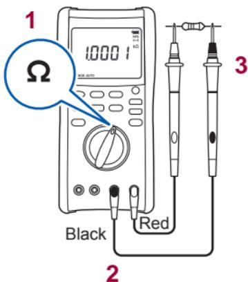
The open terminal voltage is approx. 2.5 V or less. The measurement current (DC) varies depending on the range. (p. 86)
