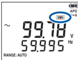
A buzzer sounds when the maximum value is updated with MAX displayed or the minimum value is updated with MIN displayed.
