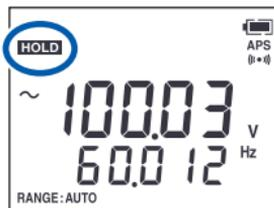
To retain the measured value, press **HOLD**. (**HOLD** lights up and the measurement value is retained.)
