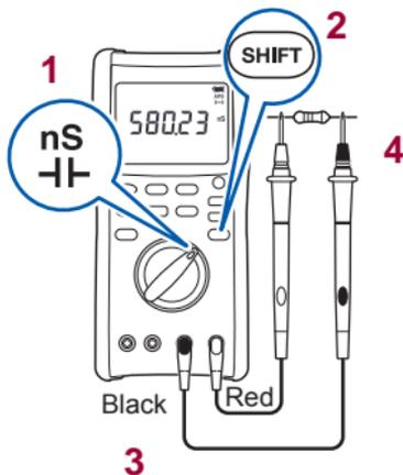
The open terminal voltage is approx. 2.5 V or less. The measurement current (DC) is approx. 96 nA. (p. 87)
