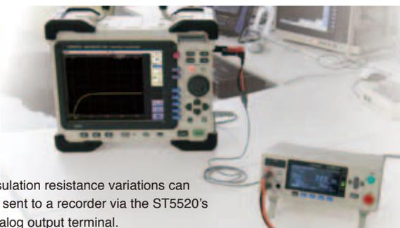
Insulation resistance variations can be sent to a recorder via the ST5520's analog output terminal.
