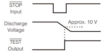
[FAST]: The signal returns to high at about the same time as the test is completed.
