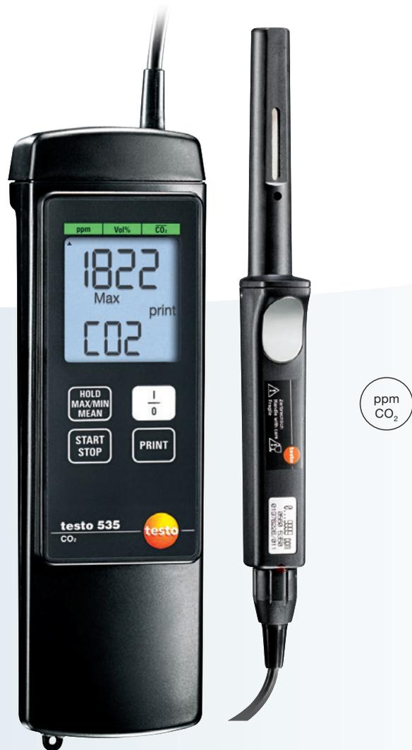
Bad air quality in indoor rooms due to excessively high CO<sub>2</sub> concentrations (greater than 1000 ppm) leads to tiredness, lack of concentration and can even cause illness. testo 535 is a precise, reliable CO<sub>2</sub> measuring instrument for monitoring Indoor Air Quality. The high-quality and stable 2-channel infrared sensor allows long-term measurements, and does not require repeated adjustment.
